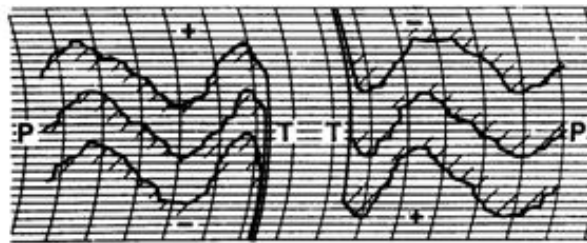
Fig.N°1- Profile error generated by the non fulfillment of the even contacts condition
